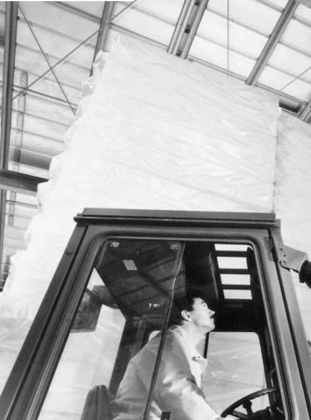
These simple-looking foam boards being stacked by Rüdiger Hahn at our site in Ludwigshafen, Germany, have a dual purpose: The BASF plastic Basotect® provides sound as well as heat insulation. It can be found in the stations of the Paris Metro.
