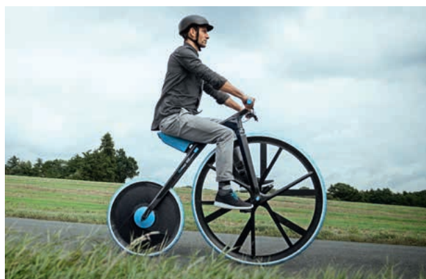
“Concept 1865” is made almost entirely of plastics from BASF. Only its brakes, axles, and motor are still made of metal.
