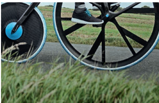
“Concept 1865” is made almost entirely of plastics from BASF. Only its brakes, axles, and motor are still made of metal.
