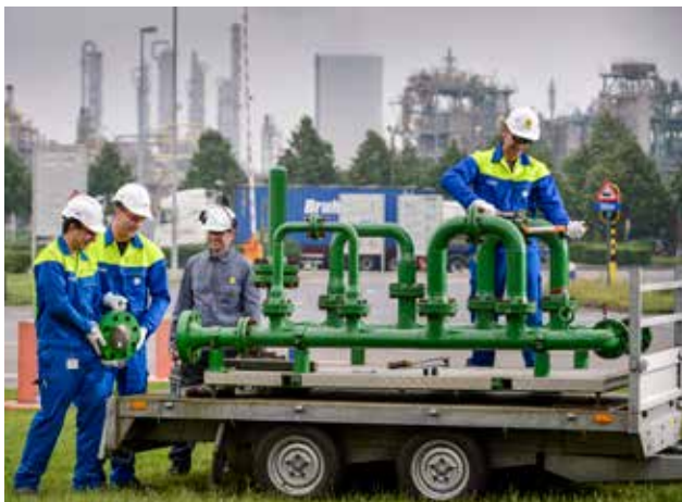
The focus is on learning by doing. Sometimes, a test set-up can be the solution, for example when learning to mount flanges.
