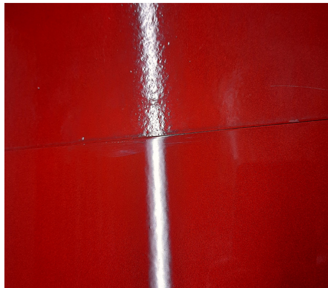
Improved appearance of Sovermol containing clear coat sprayed over a red base coat
