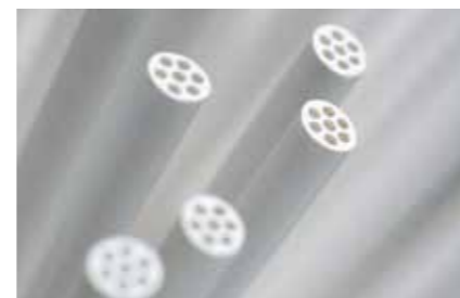
Cross-section through the filtration fibers: The honeycomb-like arrangement of the seven capillaries stabilizes the fibers. In this way the membranes are protected from fine cracks through which disease pathogens could penetrate.
