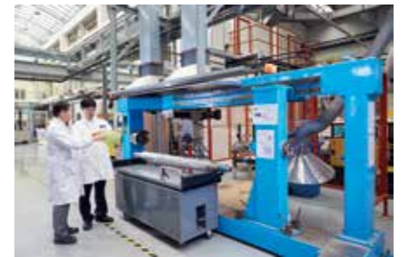
This machine will be used to test the PU filament winding process.
