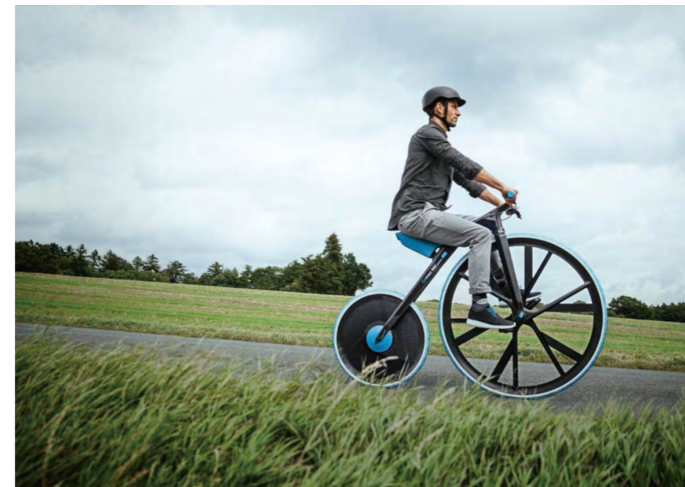
The "Concept 1865 – Rethinking Materials" e-bike utilized 24 different BASF plastics, offering up to a 60% weight reduction potential compared to their steel counterparts.
