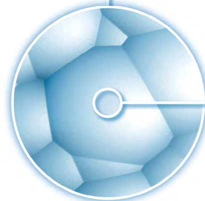
Midsole of five to ten millimeter fused foam beads made of Infinergy
