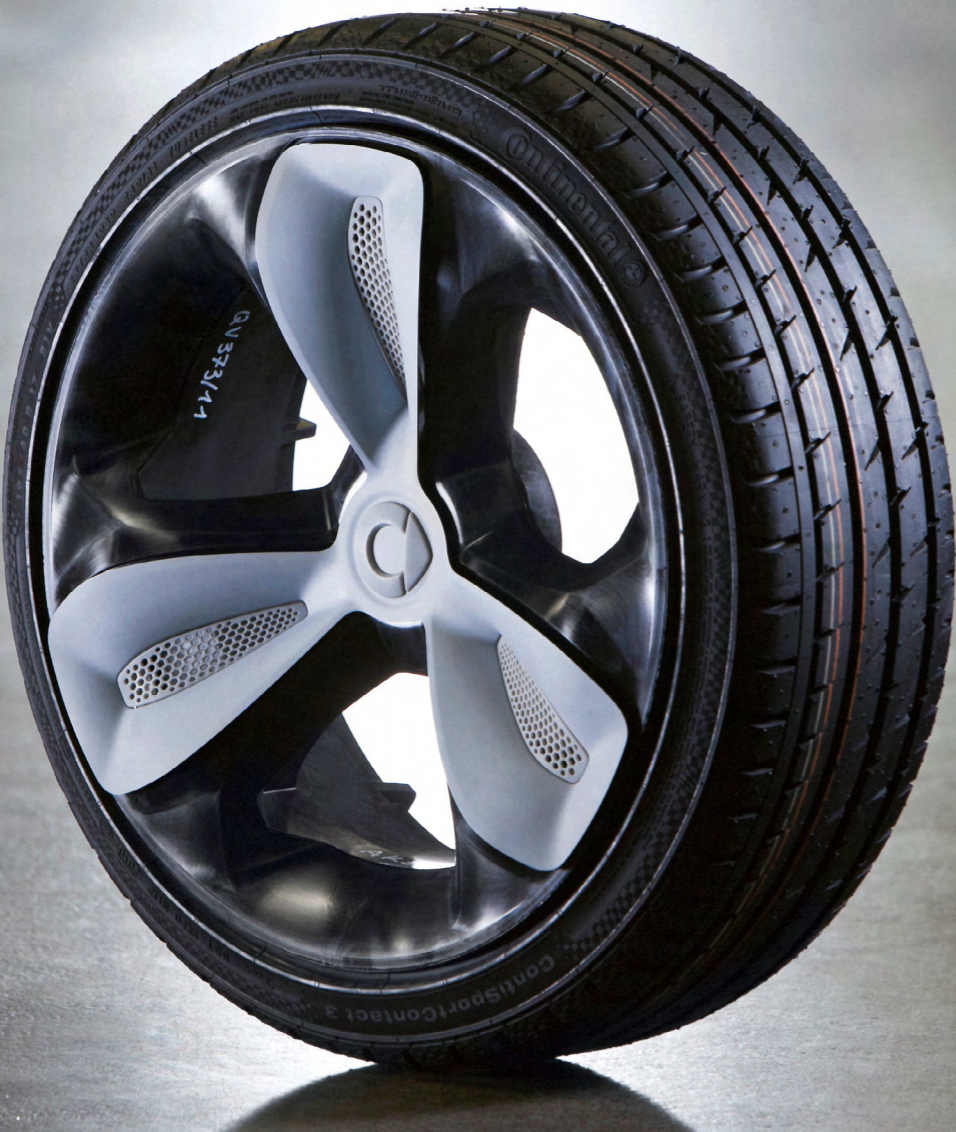
The plastic wheels on smart forvision provide an even better demonstration of the ultimate performance of engineering plastics.
