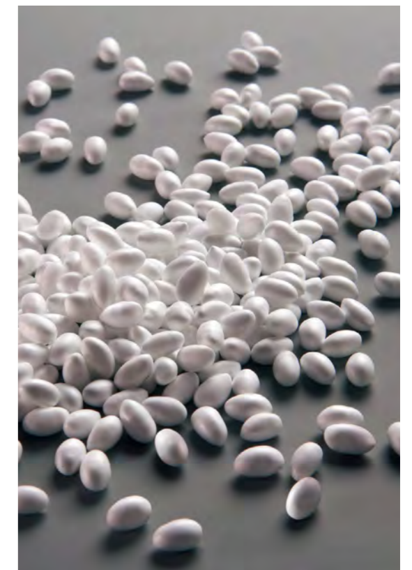
Rebound effect material: 2,500 Infinergy foam beads form the midsole of the new running shoe.
