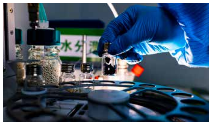
At BASF Shanshan R&D Innovation Center, an analytical technician is testing the moisture content of cathode tapes.
